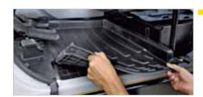
Detachable two-piece floormat with handles for easy removal. A floor drain is located under the mat to facilitate inside cab cleaning.
