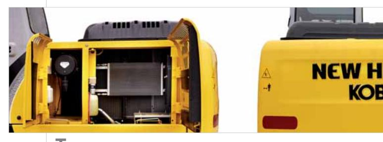
he simplified layout of all vital components of the New Holland E175B under both the right and the left side panels makes maintenance much easier, less time consuming and less costly, and provides much better access for servicing. There is plenty of room in all compartments and most components are positioned in such a way to enable easy access from ground level. **An elegant and modern design added to state-of-the-art technology.**
