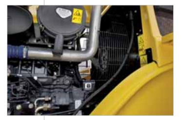
A variable speed hydrostatic fan, automatically actuated by a thermostatic sensor, with eight plastic blades, draws fresh and clean air from outside through the radiators and the hydraulic oil tank.
